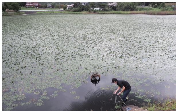
▲ Measuring water quality with analytical equipment at an agricultural pond
